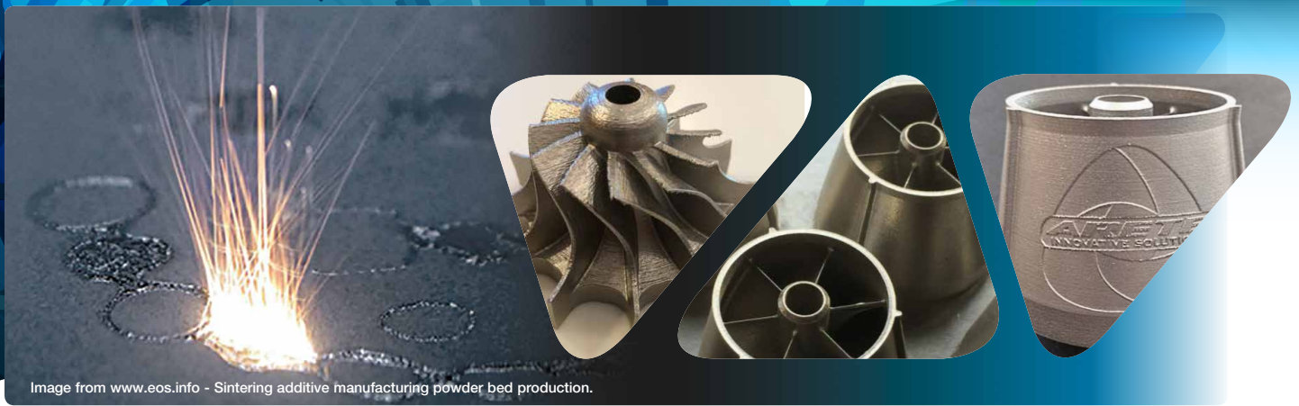
Image from www.eos.info - Sintering additive manufacturing powder bed production.
